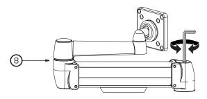
Position Arm so it is parallel to desk surface. Turn bolt clock wise for lighter monitors.
