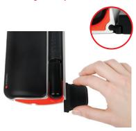
Fit the end of the short riser 3 into the slot on the back of the RollerMouse unit.
