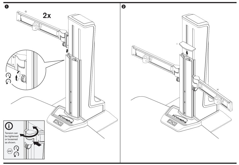
2 3 **2**x **2**x Tension can be tightened or loosened as shown. **2**x
